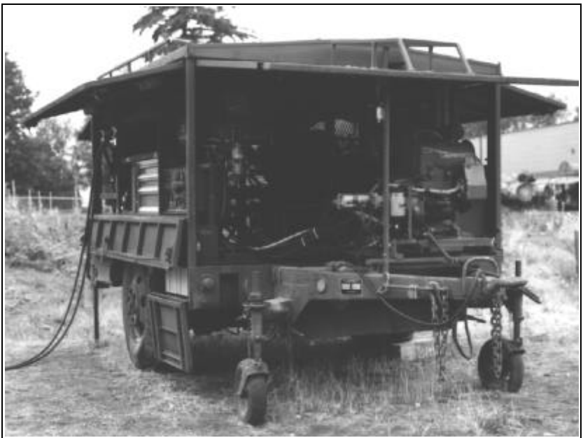
Fig 6-3-1 Trailer Mounted Hydraulic Tool System – Open Configuration
