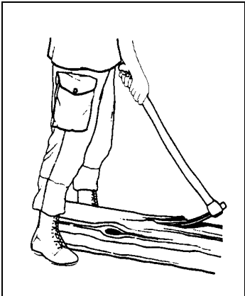
Fig 3-3-7 Correct Method of Using an Adze
